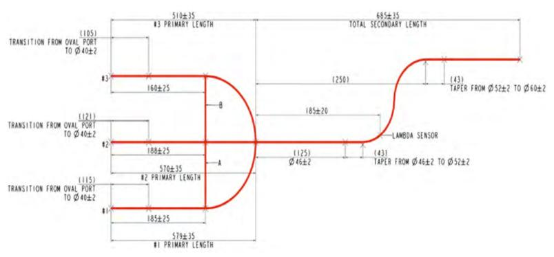
• All pipe diameters shown are internal diameters.
