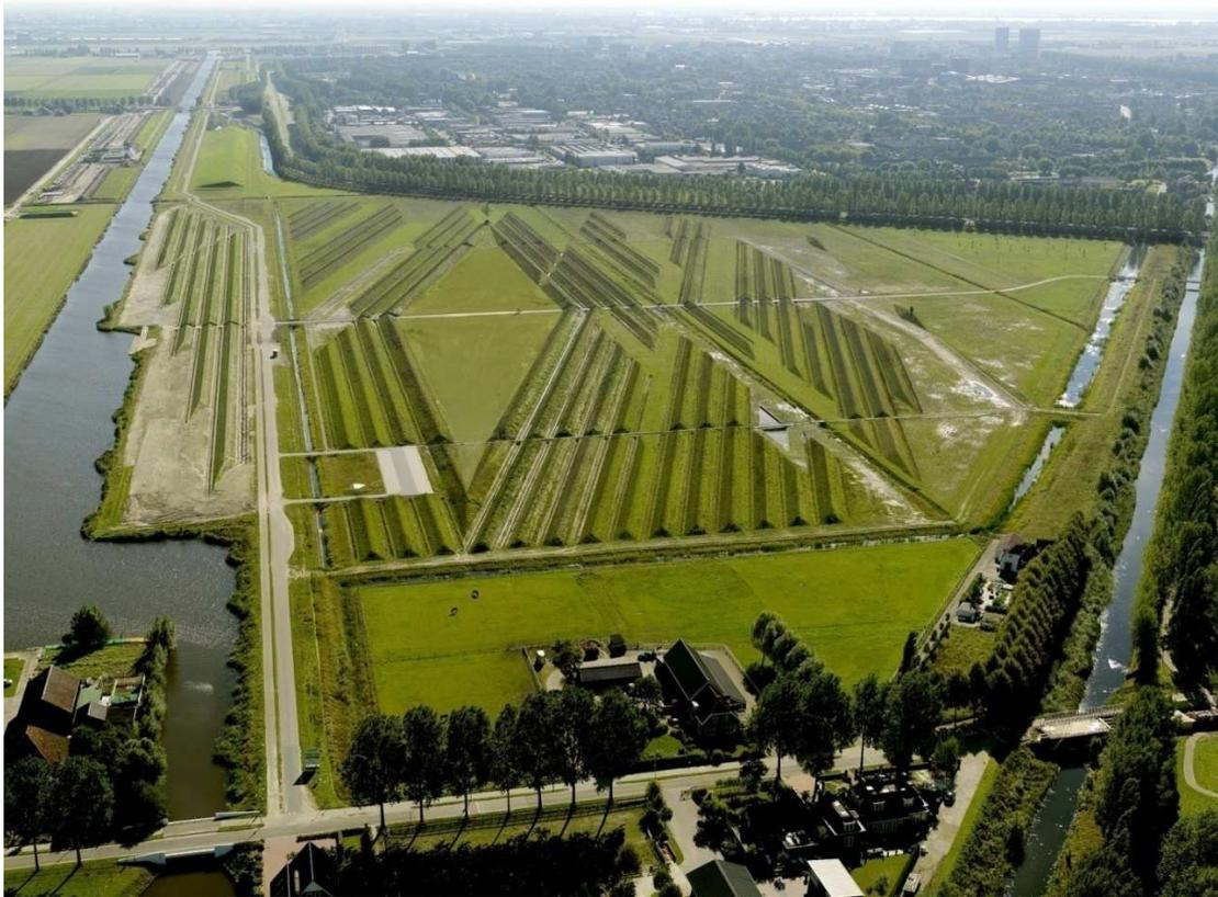
This goal, has been obtained by means of earth embankments lined perpendicular in respect of the sound waves creating a certain number of oblique planes able to distort and disperse the sound and lowering in this way the sound level on the residential area as shown in the following scheme.
