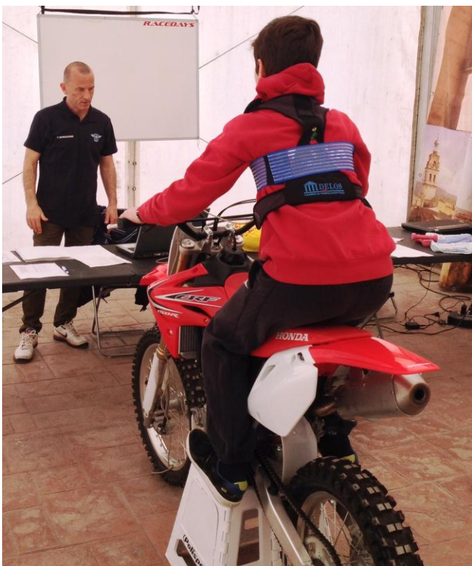
Fig. 4 - Resistance for keeping the riding position on the bike with bent knee legs with vertical controller
