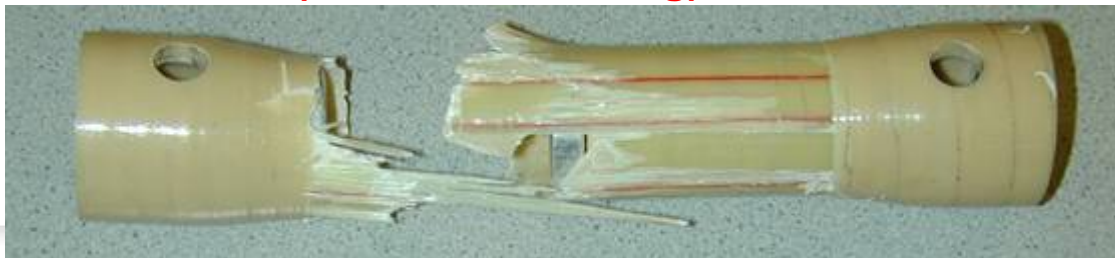
broken femur (test without airbag)
