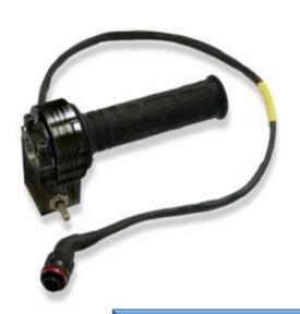
Sophisticated engine management systems controlling the throttle with electrical motors. The driver intention is coming from the throttle grip by sensor signals. This type of control was introduced on cars many year before PTWs. Because in racing carburetors have been used much longer, this development was delayed for years. With the limitation of fuel consumption and to achieve a maximum of drivability drive by wire is now in racing as well.
